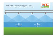
The entirely new design of the Syngenta XC Turf Nozzle has been developed with a unique orifice shape that assures even coverage, even where nozzle spraving height is reduced over undulating ground.
