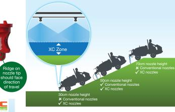
Wider spread + even droplet distribution = more consistent coverage at nozzle heights down to S0cm
